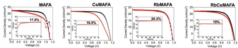
Figure 2 J-V curves illustrating hysteresis reduction with the addition of Rb<sup>2</sup>
