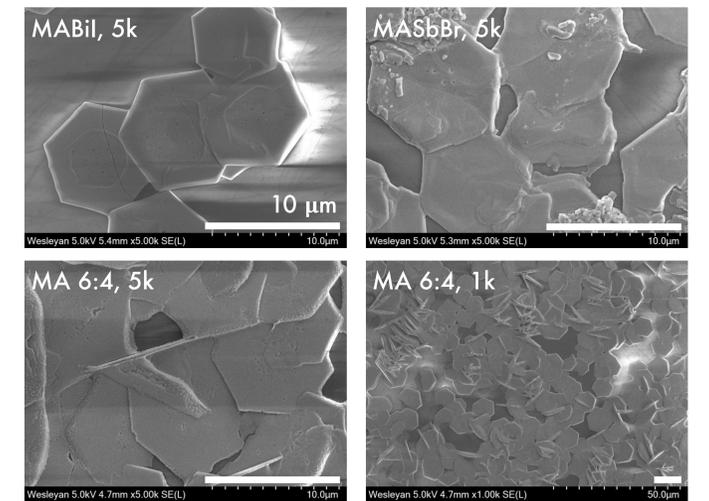
Figure 7 SEM images of our three lead-free samples at 5k magnification, as well as our hybrid sample at 1k to illustrate structure on a larger scale
