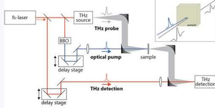
Fig. 2 Time-resolved terahertz spectroscopy (TRTS) set-up.
